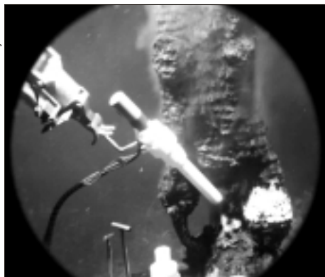
Nearly 2 miles under the ocean, a wand extended from the submersible Alvin houses a thermometer, electrodes for chemical measurements, and a biosipper to collect water samples for in situ analysis. The in situ data help scientists understand the chemical and biological processes as they occur near deep-sea hydrothermal vents.
